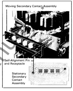
Secondary contacts having a maximum of 48 points are located at the rear of the draw-out element. Engagement of secondary contacts is assured by automatic selfalignment and positive contact of mating parts.
