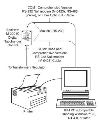
Figure 1 Direct Connection
