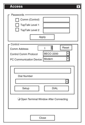
Figure 9-11 Communication Access (Modem) Dialog
