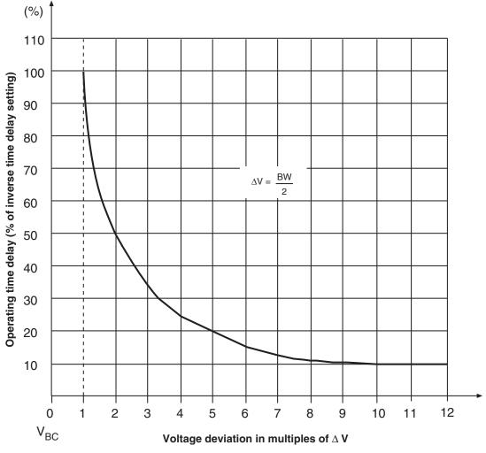
Figure 3-1 Inverse Time Delay Curve
