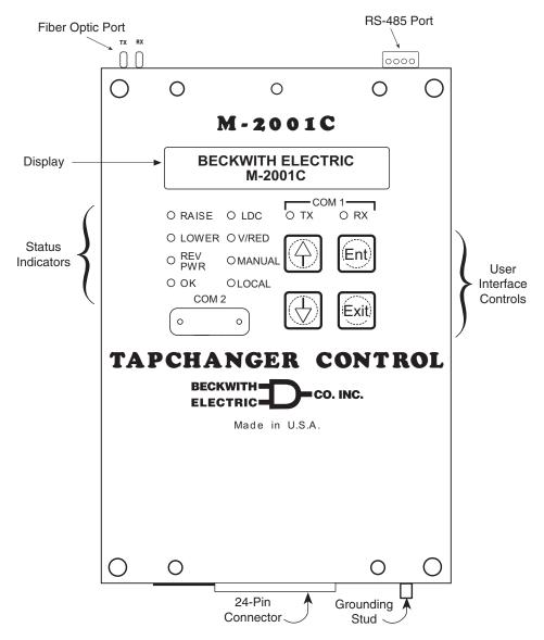
Figure 2-1 M-2001C (BASE-RS) Tapchanger Control
