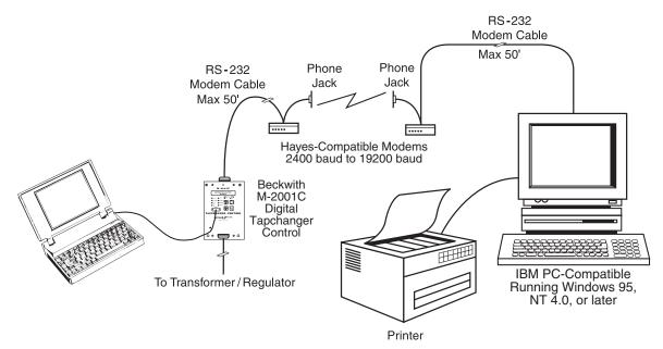
Figure 2 Modem Connection
