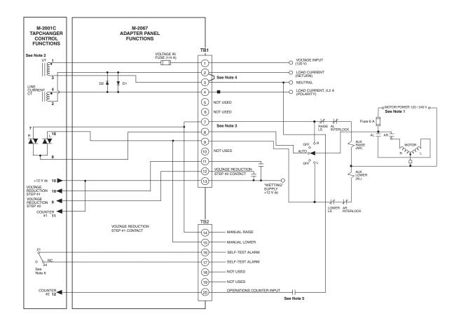
• WARNING: In no case should the line current circuit be interrupted with the regulator or transformer energized. Do not remove auxiliary current transformers without shorting the current inputs. Death or severe electrical shock can occur.
