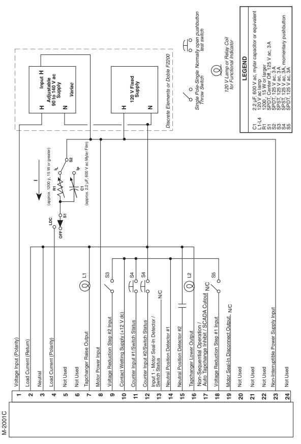
Figure 7-1 External Connections for Test Procedure
