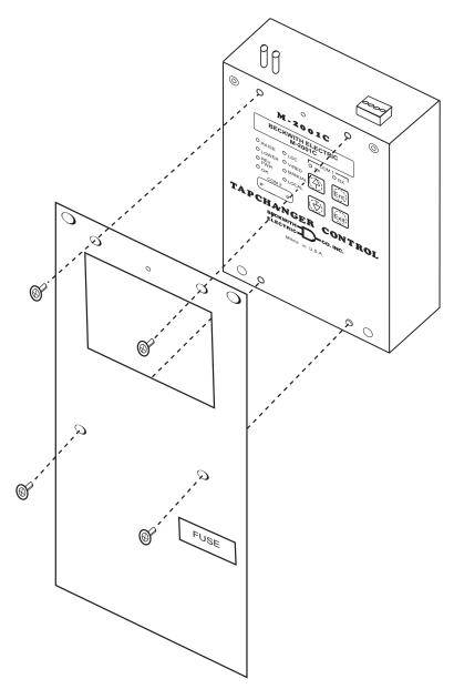
Figure 1-2 Typical Adapter Panel Mounting
