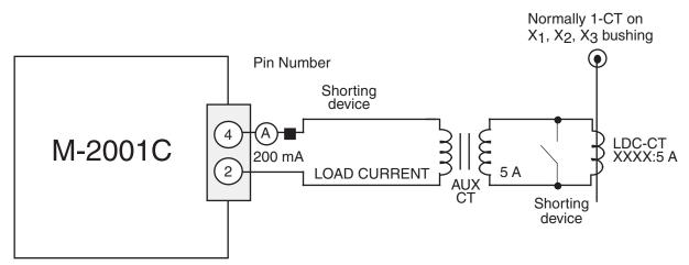
■ NOTE: Pin numbers indicated above are accurate for the M-2050 Mounting Kit only; check the Application Guide of the specific adapter panel used for proper pin numbers.
