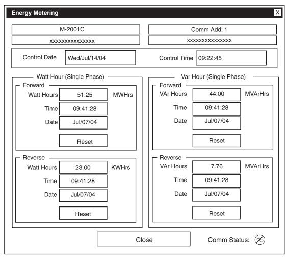
Figure 9-24 Energy Metering Screen
