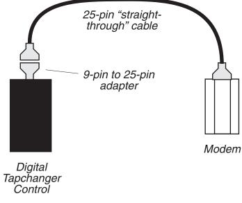
Figure 9-38 Modem Cable 9-Pin to 25-Pin
