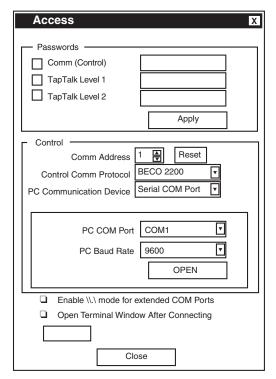
Figure 9-10 Communication Access (Serial) Dialog
