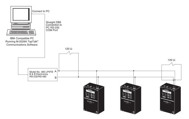
Figure 5 RS-485 Network Connection
