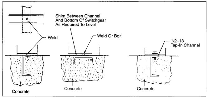
Figure 21: Switchgear mounting floor channels
