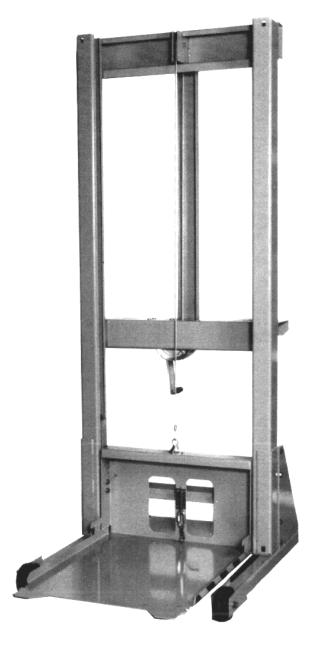
Figure 29: Circuit breaker lift truck
