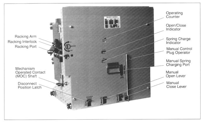
Figure 10: Vacuum circuit breaker Type VAD-3
