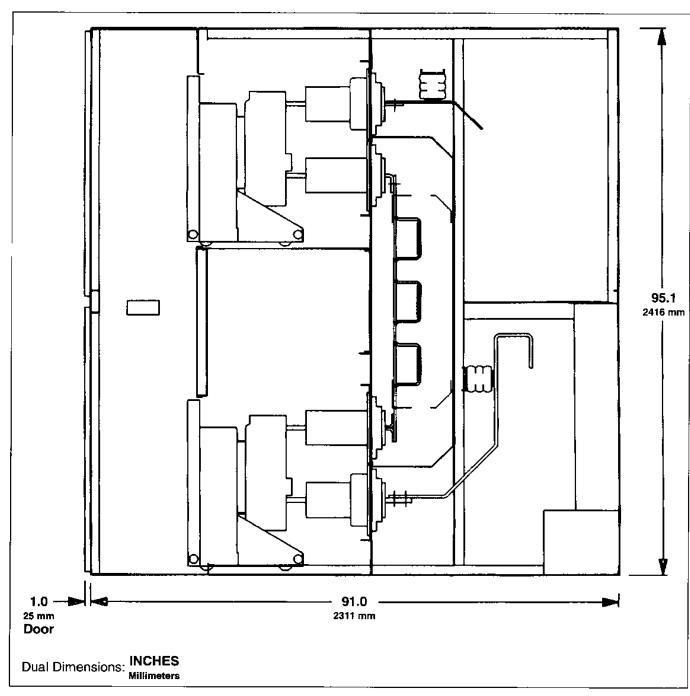
Figure 31: Series 3 Metal-clad indoor switchgear outline
