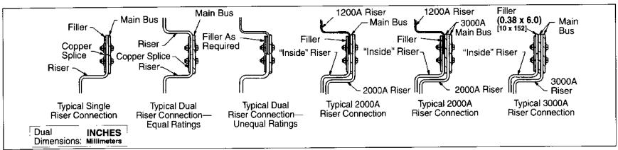
Figure 24: Main bus connections—side view
