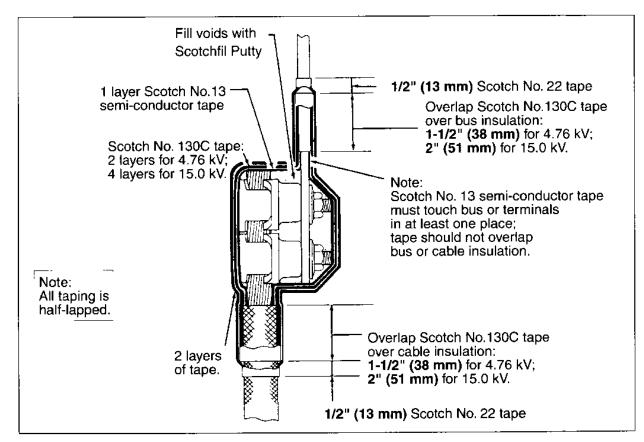
Figure 28: High voltage cable lug insulation
