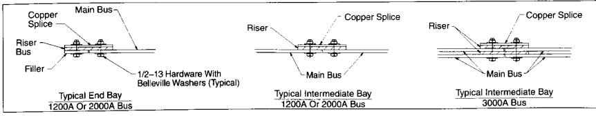
Figure 25: Main bus connections—top view
