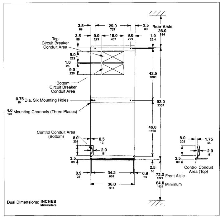
Figure 22: Floor plan
