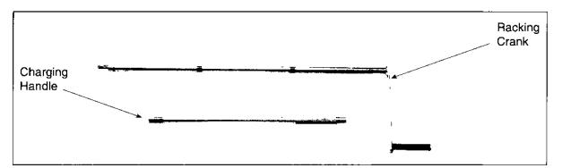
Figure 20: Circuit breaker racking and charging handles
