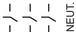
Four-wire SN, 240 Volts AC, No Fuse
