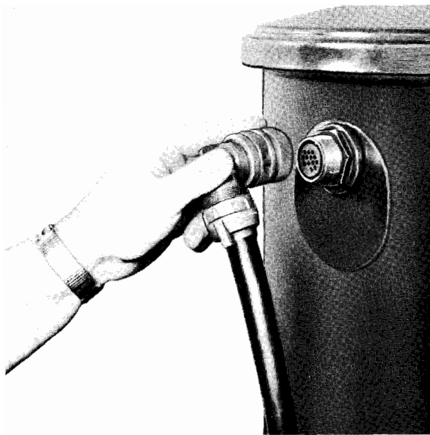
Fig. 11 - Disconnecting Flexible Cable from Regulator Tank
