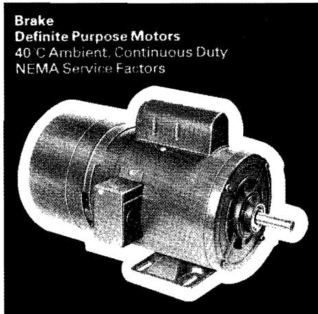
A line of single phase and polyphase motors equipped with a magnetic brake. The brake torque on each rating is three pound-feet continuous. Motors are available as rigid mounted or round frame with NEMA C flange mounting. The NEMA service factors, shown in the table below, for open motors enables them to carry small overloads continuously. Enclosed motors have a service factor of 1.00.
