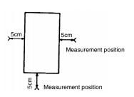
The inverter is a heat-emitting body. Make sure to provide proper space and ventilation when installing in the cabinet. When installing inside a cabinet, we recommend peel of the top seal although 40°C or less.
