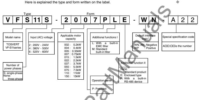
\* This code represents the factory default logic setting. You can switch from one input/output logic to the other using slide switch SW1. (See 2.3.2)
