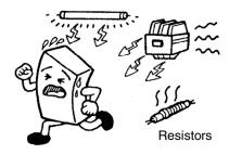
Solenoids:Attach surge suppressor on coil.Brakes:Attach surge suppressor on coil.Magnetic contactors:Attach surge suppressor on coil.Fluorescent lights:Attach surge suppressor on coil.Resistors:Place far away from VF-S11 Inverter.
