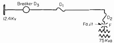
Short circuit current for fault at F is 500 amperes. Full load current for 75 kva transformer is 6.0 amperes.
