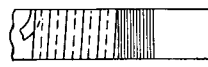
FINISHED LAYER HALF-LAPPED COTTON TAPE CORD OR SEW ENDS TAP- ING FOR PERMANENT FASTENING OR TAPE WITH FRICTION TAPE
