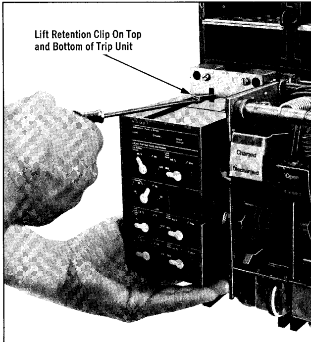
Fig. 39 Removing Trip Unit from Breaker.
