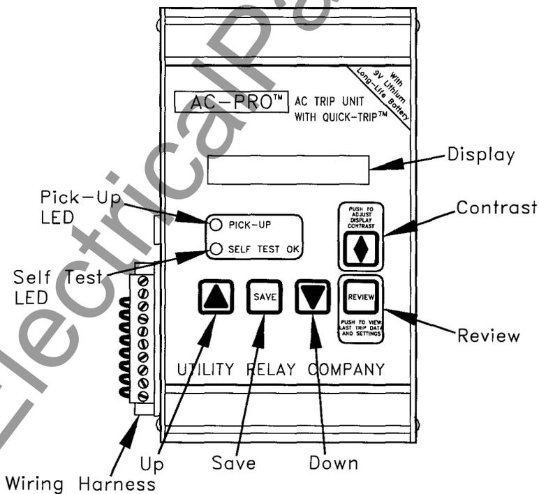
Figure 5.2 AC-PRO™ Vertical Front View
