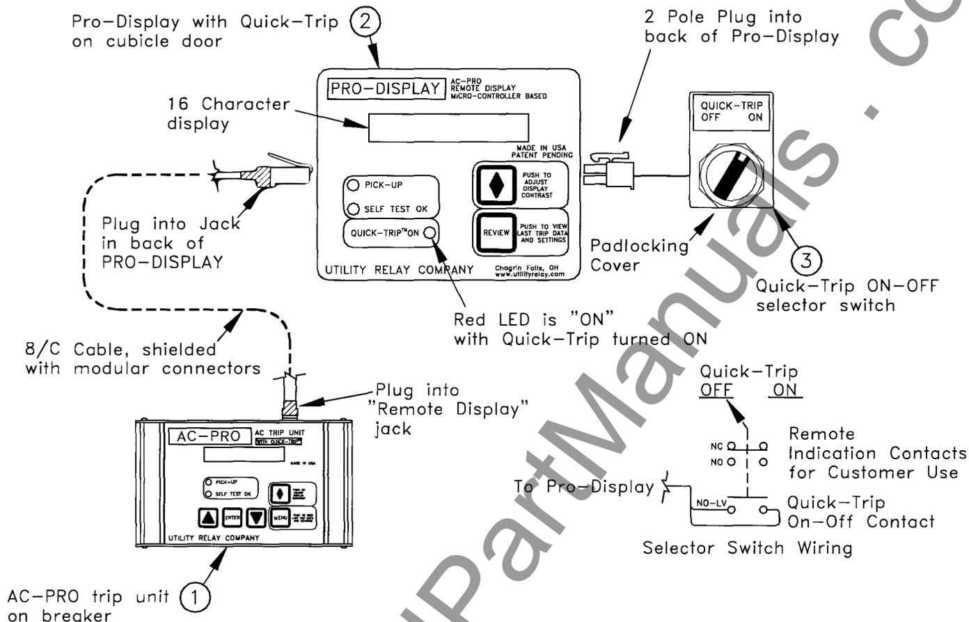
Figure 6.1 QUICK-TRIP™ Connections
