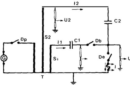
Figure 3. - Diagram of synthetic circuit for line-charging current breaking tests.
