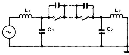
Figure 6. - Diagram of circuit for inductive current breaking tests.
