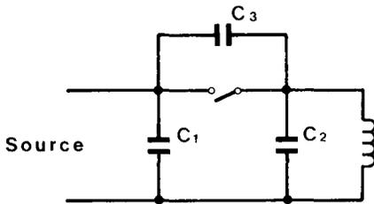
Figure 12. - Representative diagram of an inductive current interruption.
