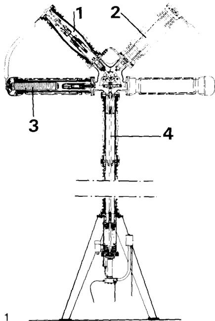
Fig. 1. - Sectional view of a pole unit of 525 kV circuit-breaker equipped with closing resistors.
