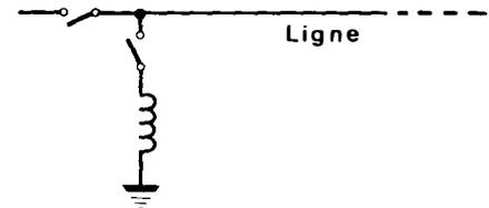
Figure 5. - Connection diagram of shunt reactors.
