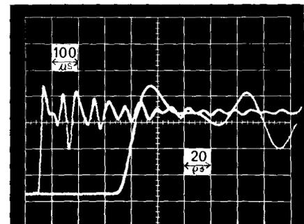
Figure 9. – Oscillogram of the TRV recorded during the interruption of a fault on the secondary side of a 220/60 kV transformer.
