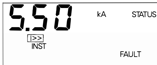
Figure 61. Trip Unit status display for instantaneous overcurrent trip.
