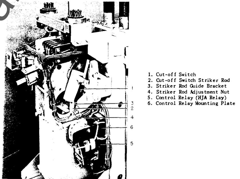
Fig. 5 Side View of Control Relay and Cut-off Switch Assembly
