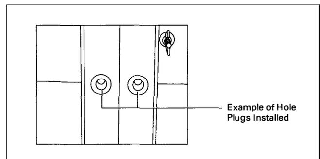
**Figure 12. Hole Plugs Installed**
