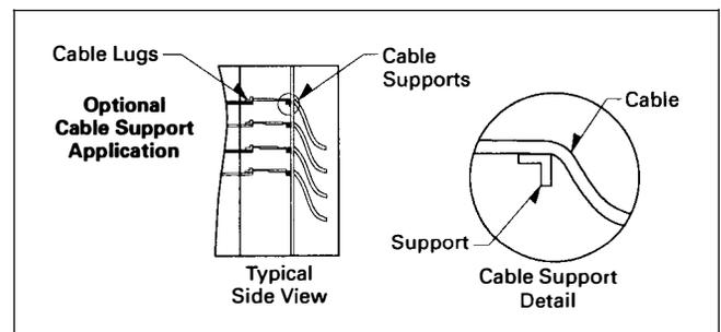
Figure 21. Cable Bracing
