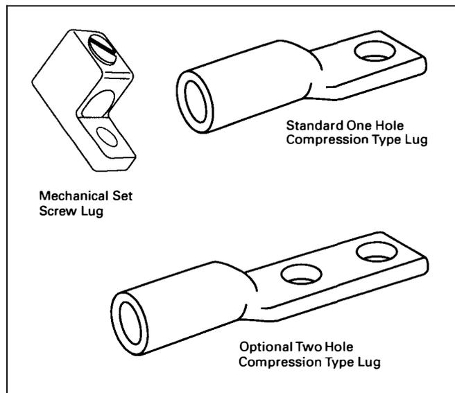
Figure 19. Screw and Compression Lugs
