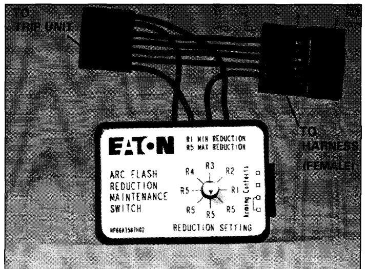
Figure 9. Connectors on the Arcflash Reduction Maintenance Switch Harness.
