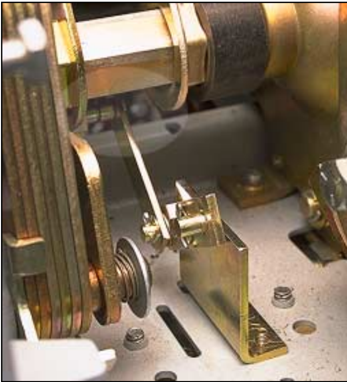
Fig. 31 Reset Pivot Assembly Arm Attached to the Breaker Jack Shaft Pin.
