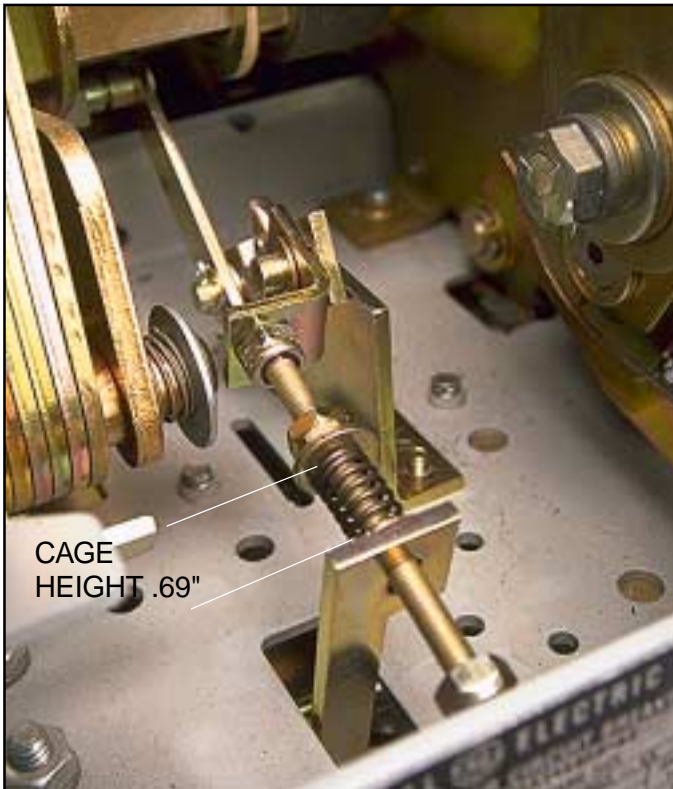
Fig. 36 Adjusting the Cage Height.
