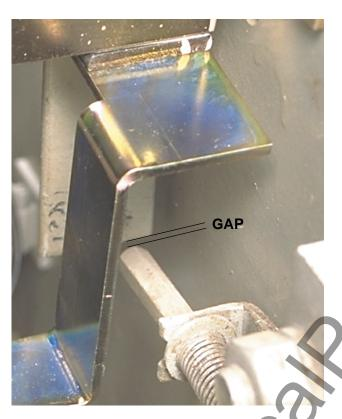
Step 8: Installing the DTA, Reset Arm, and Trip Link Assemblies
