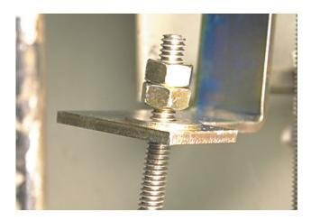
D. Align the holes in the DTA Assembly with the holes drilled in the right Breaker Side Plate in Step 3-B. Secure the DTA Assembly to the right Breaker Side Plate using the (2) .250-20 x .750' screws, (2) lock washers, and flat washers provided.
