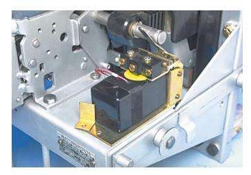
A. Remove the Tru-Arc circle clip from the right end of the Breaker Cross Bar. Slide the tubular brass spacer provided over the cross bar until it is snug against the insulating link. Re-install the circle clip.
