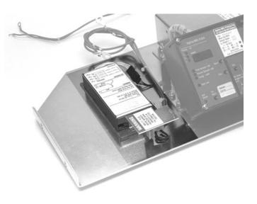
F. For Kits Supplied With a PT Module Only. Plug the connector of the PT Extension Harness into the receptacle on the PT Harness. Route the PT Extension Harness between the Aux. CT Module and the Trip Unit Assembly.
