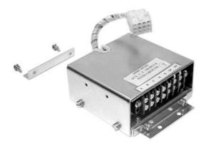
B. Using the .190" screws (4" long), lock washers, flat washers, and nuts provided, mount the Trip Unit Mounting Brackets to the Trip Unit as shown. Note the Mounting Brackets are to be installed with the holes towards the bottom of the Trip Unit. Also note that the screws, with flat washers installed, are inserted from the bottom of the Trip Unit and the flat washers, lock washers, and nuts are installed from the top.
