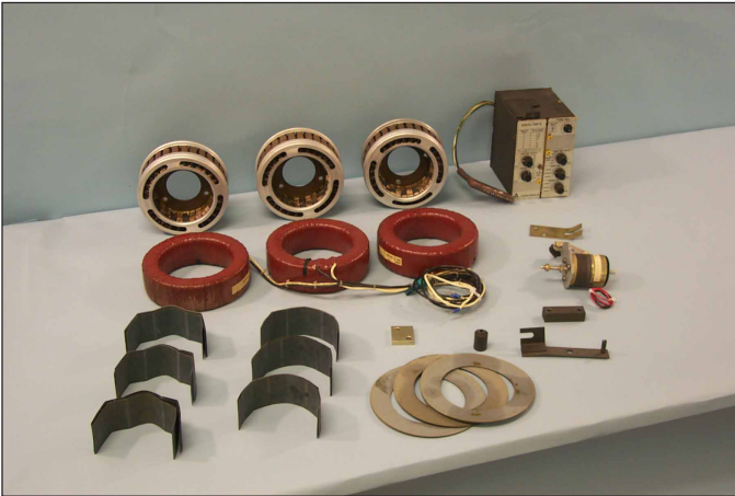
Fig. 1 Overview: Original Components Removed from the Breaker.
