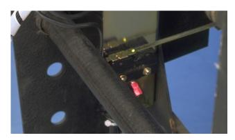
G. Use the wire ties and wire clamps provided to dress all wires and harnesses to keep them away from any moving parts within the Breaker.
