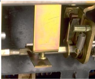
E. Remove the flange nut from the end of the DTA Shaft. Insert the Reset Arm through the existing cut-out in the Breaker Shelf then attach the Reset Arm to the DTA Assembly using the pivot pin and (2) "X" washers supplied. Apply Loc-Tite® 242 to the threads of the DTA Shaft then reinstall the flange nut.
