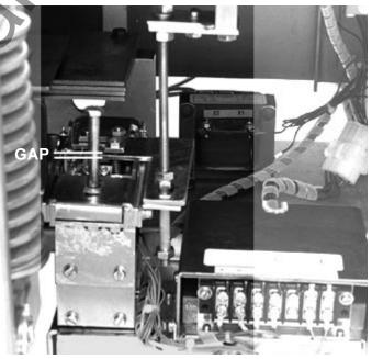
F. The gap between the adjusting screw on the left side of the DTA Assembly and the rear of the Breaker Trip Bar should also be .06". Adjust the gap by loosening the lock nut and turning the adjusting screw until the gap is achieved. Apply Loc-Tite® 242 to the threads of the adjusting screw then retighten the lock nut.
