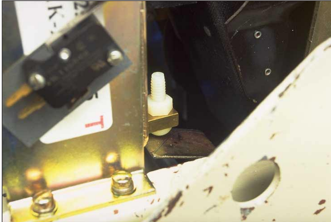
Fig. 40 Correct Position of the Trip Paddle
