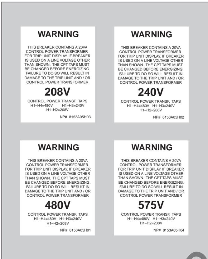
Fig. 34 CPT Voltage Labels supplied with the CPT Kit.
