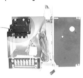
A. Align the holes in the base of the Breaker Mounted CPT with the holes in the Trip Unit Mounting Bracket as shown. Secure the CPT to the Trip Unit Assembly using the using the (4) .190-32 x .500" screws, (8) flat washers, (4) lock washers, and (4) nuts supplied.
