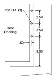
B. Align the Trip Unit Assembly with the holes just drilled. Secure the Trip Unit Assembly to the Breaker Front Plate, as shown, using the (3) .250-20 x .750" hex bolts, (3) lock washers, and (3) flat washers supplied.
