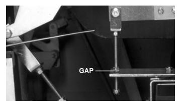
B. Loosen the lock nuts on the Reset Shaft, below and above the brass spacer. Turn the adjusting nuts until a cage height of approximately .73" to .77" at the centerline of the Reset Shaft is achieved. Tighten the lock nuts.
