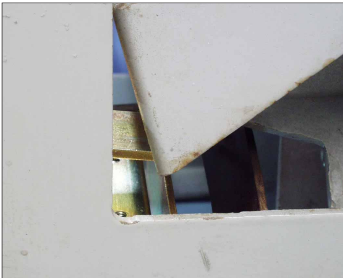
Fig. 13 Correct Orientation of the DTA Reset Arm
