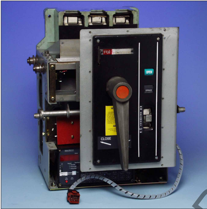
Fig. 59 Original Front Components Reinstalled on the Breaker
