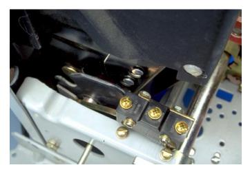
A. Using Drilling Plan B, drill two (2) .219" diameter holes in the top of the left Breaker Frame.
