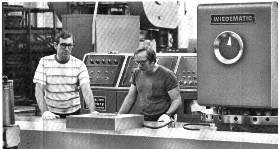
Computerized tape controlled presses are used to accurately fabricate switchgear panels and subassembly parts.
