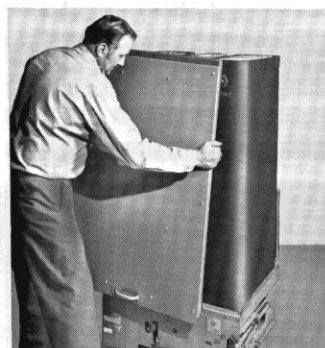
Removing the front shield. Merely loosen two screws and
