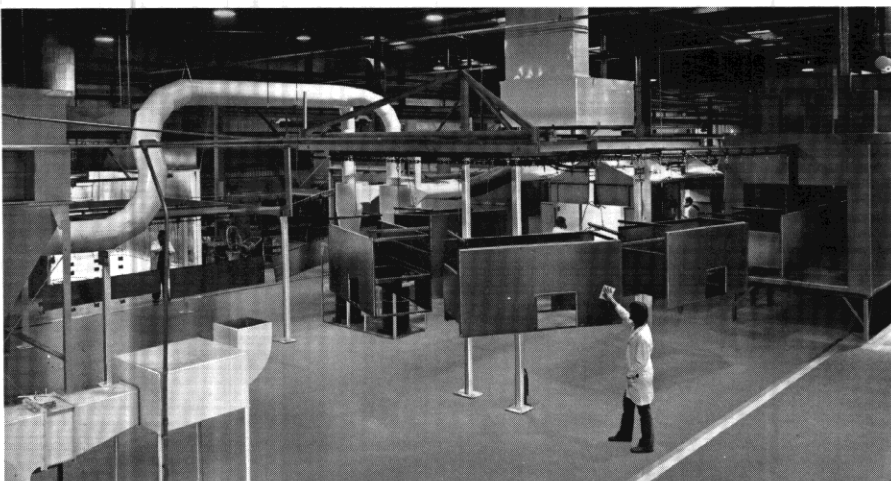
Latest multi-stage cleaning and painting equipment operating under controlled standards provide uniform paint thickness on all parts.
