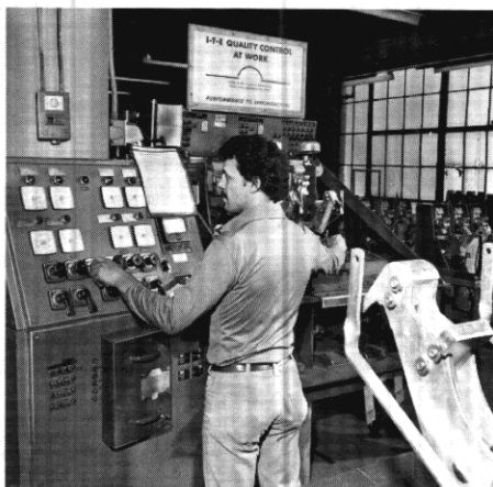
Each circuit breaker manufactured is tested in special fixtures to assure dimensional accuracy and proper alignment of circuit breaker with the switchgear.
