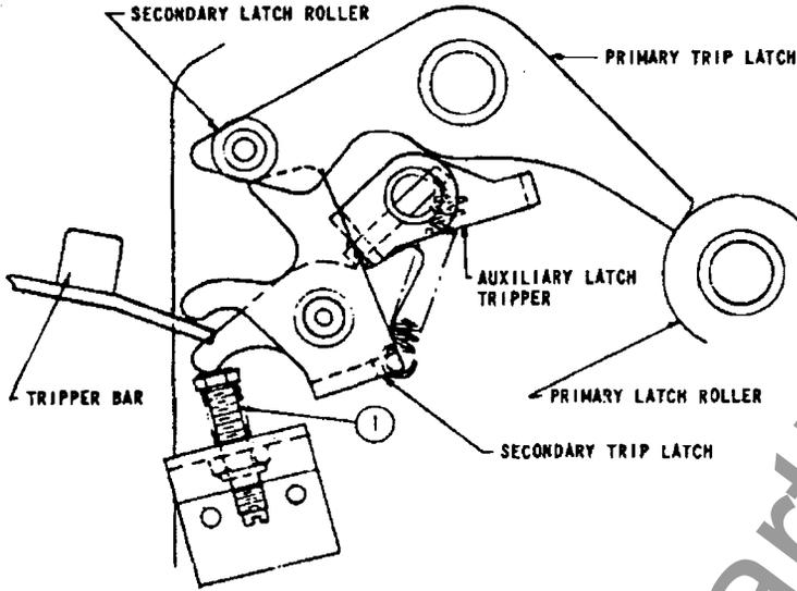
Fig. 5 — Primary Trip Latch Adjustment
