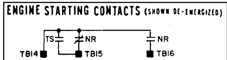
Figure 1-4. Engine starting contact label and locations for 260 - 4000 amp switches.
