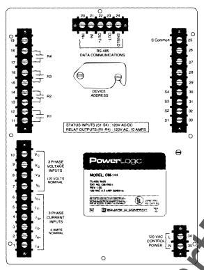
Circuit Monitor with 4 Status Inputs, 4 Relay Outputs (Models CM-144, CM-244)
