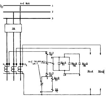
Fig. 6 (K-6375669-6) External Connections of Three Type IAC51R Relays used for 3-Phase Circuit Protection.
