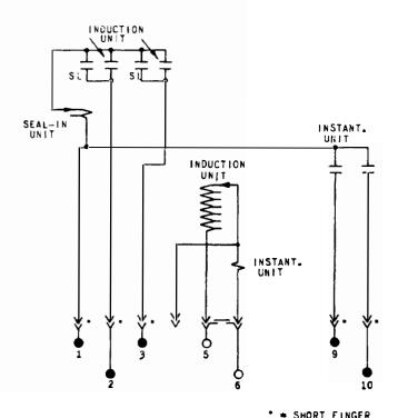
Fig. 15 (K-6209663 [8]) Internal Connections for the Type IAC52B Relay (Front View)
