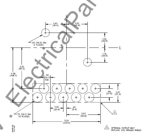
Figure 4-5. Panel Drilling Diagram S1 Case, (Projection Mount)
