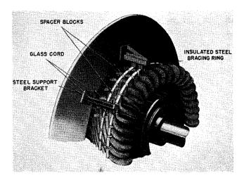
FIG. 4. Stator Winding End Turn Bracing
