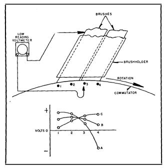
FIG. 28. Adjustment of Commutating-Pole Field Strength
