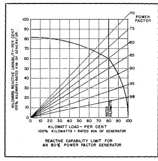
FIG. 24. Reactive Capability Curve
