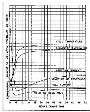
FIG. 23. Typical Insulation Resistance Curve
