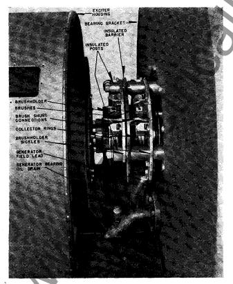
FIG. 9. Exciter Housing Rolled Back Giving Access to Collector
