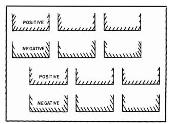
FIG. 27. Correct Method of Staggering Brushes
