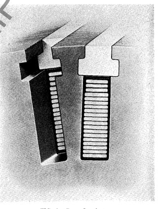
FIG. 6. Rotor Insulation.
