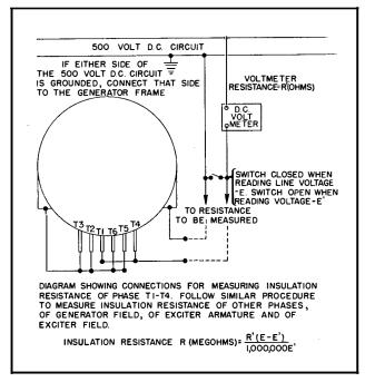
FIG. 21. Connections for Insulation Resistance Measurement
