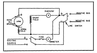
FIG. 29. Connections for Restoration of Residual Magnetism of Exciter
