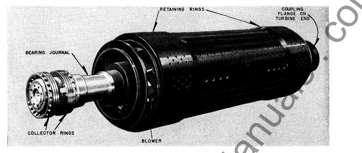
FIG. 5. Complete Rotor
