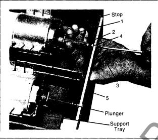
Figure 10. Adjustment of the Plunger
