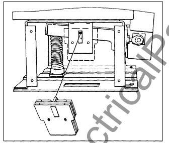
Figure 18. Auxiliary Contact Block Replacement
