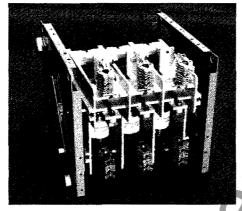
Three pole reversing contactor with line and load fingers, includes mechanical interlock arm for mechanical interlock, 120 volt coil (used as reversing contactor or reactor shorting contactor of a reactor reduced voltage starter)
