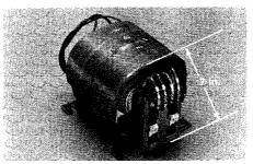
2 KVA control transformer 2300/240/120 volt, 60 Hz **Style No. 2147A11G02** 4160/240/120 volt, 60 Hz
