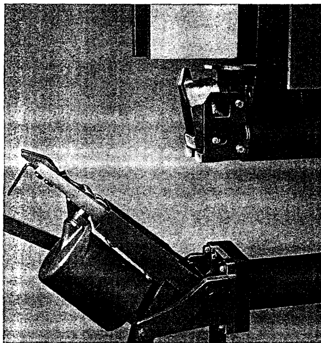
Fig. 94. Main and auxiliary contacts.
