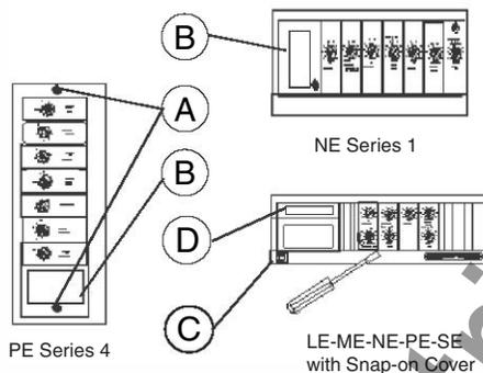
**Figure 8: Screw Retained and Snap-On Unit Covers**
