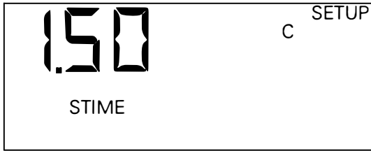
Figure 11. Trip unit display for short-time pickup.
