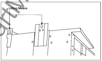
Figure 2. Typical Outdoor Lifting Means
