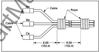
Figure 20. Cable Bracing
