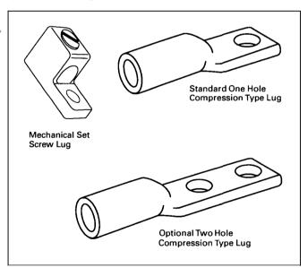
Figure 19. Screw and Compression Lugs
