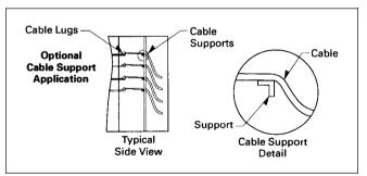
Figure 21. Cable Bracing
