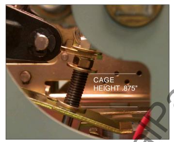
Fig. 49 Proper Cage Height Adjustment.
