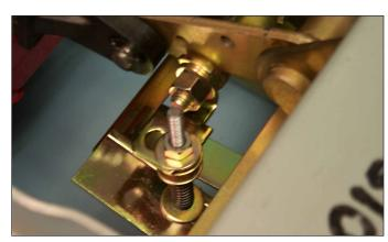
Fig. 48 Reset "L" Bracket Installed on the DTA Shaft.
