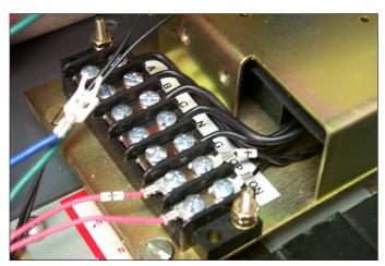
Fig. 57 DTA Wires Connected to the Aux. CT Module Terminal Block.
