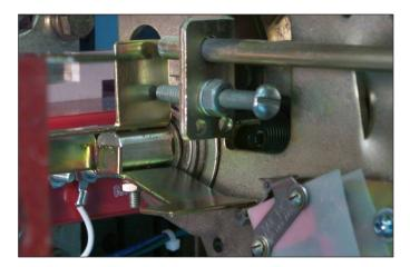
Fig. 41 Trip Finger Installed on a Short Trip Shaft.
