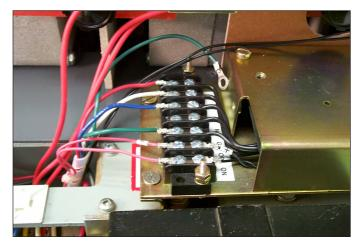
Fig. 58 Sensor Harness Connected to the Aux. CT Module Terminal Block.
