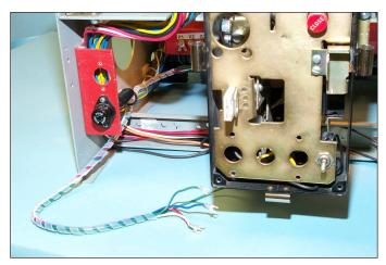
Fig. 11 Routing of the Sensor Harness.
