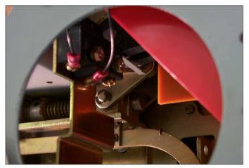
Fig. 63 External Harness Wires Connected to the Auxiliary Switch.
