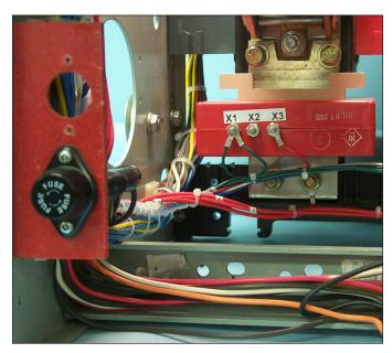
Fig. 17 PT Wires Secured to the Sensor Harness.
