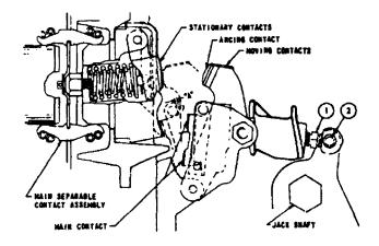
Fig. 3 — Contact Pressure Check and Adjustment
