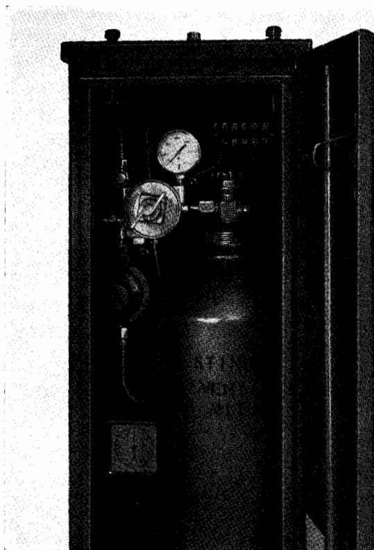
FIG. 5. Reducing Valve on Nitrogen Cylinder
