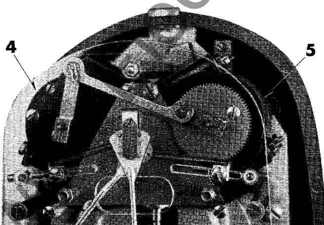
Close-up view of thermal elements and linkage mechanism.
