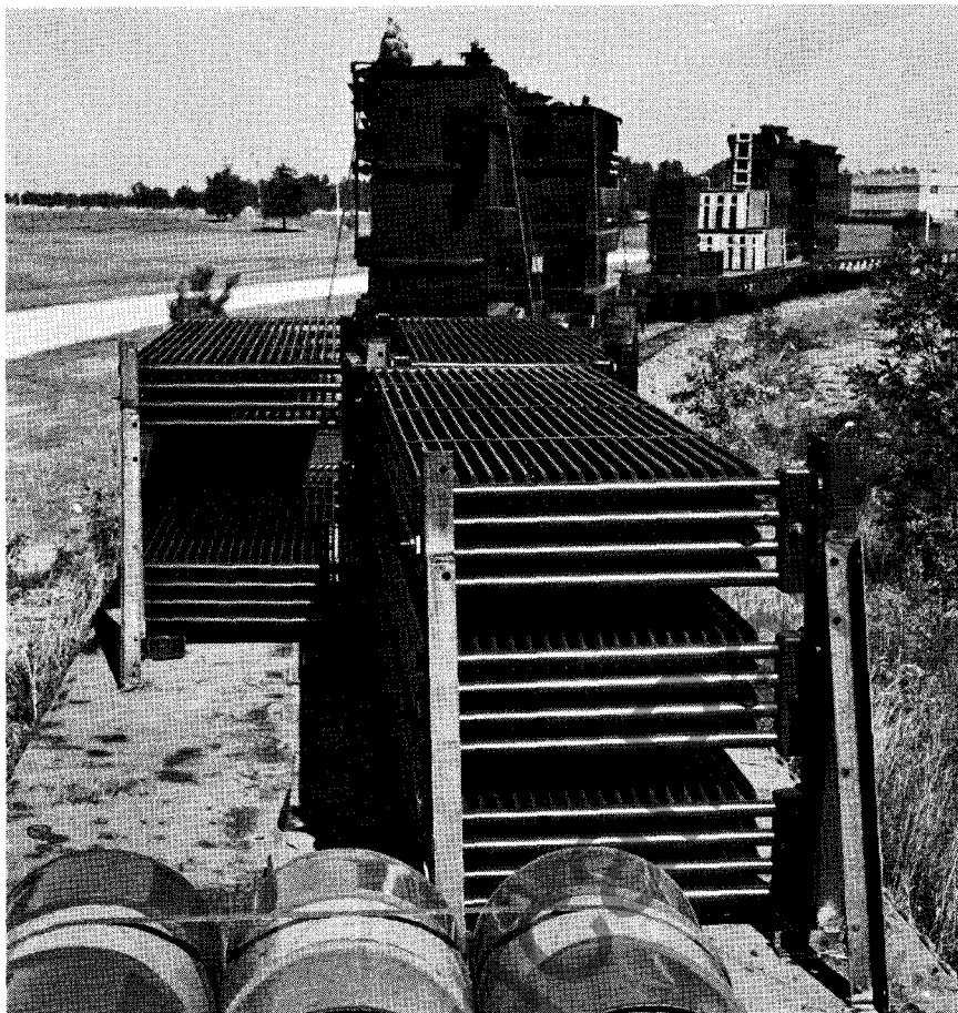
Fig. 1. Method of loading radiators for shipment
