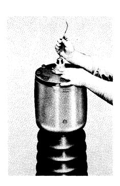
D. Assembly of the pin to hold the transformer lead in place
