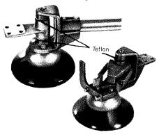
The use of TEFLON on the bushings of the live side bearings provides long life, low friction operation, and eliminating of all lubricants.
