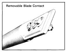
The blade tip contact is removable hot tinned copper with heavy silver plated strips on contact surfaces. Blade tip is held in position with stainless steel bolts.
