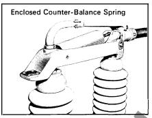
The spring, for counter-balancing the weight of the blade, is completely enclosed in the hinge assembly. This gives protection from ice buildup or other forms of mechanical interference. (No counterbalance for 115 Kv, 600 amp.)
